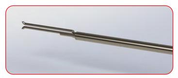
In its standard version, the CP2 is composed of a Pitot tube and a thermocouple, however, it is possible to upgrade this version with a 25mm filterholder or sintered filter to use it also as sampling solutions in small stacks for particulate matter or gas sampling.
